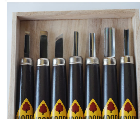
A seven tool set, with a variety of tools, all of which are useful to complete mokuhanga. This set has the knife tool, three sizes of gouge, two flat chisels and a v-gouge.
