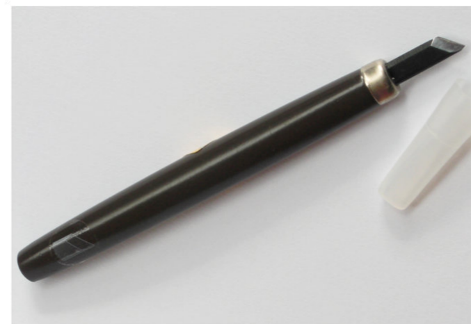
Above: the knife tool, which has an angled bevel. This is a right-hand tool and left-hand tools are also available.
